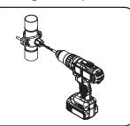
3. For the standard faucets drill a 1/4" hole through one side of the pipe. The drill should be kept straight and centered to avoid damaging the saddle valve. Do not drill through both sides of the pipe!
