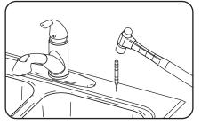
2. Center punch hole to provide a starting point for your drill.
