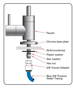
Take length of 3/8" blue tube and make sure it is has a fresh cut and is free of foreign materials and any scratches on the outside surface. Install the tubing into the push in type fitting at the base of the faucet. Make certain that it is inserted all the way in; once inserted give it a slight pull to make sure it is locked into the fitting.
