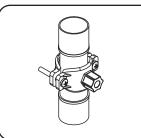
2. Tighten the clamps with the help of the two bolts.
