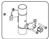
1. Install the drain saddle valve on to the drain pipe. Use 1/4" saddle for drain water line.
