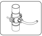
4. Attach 1/4" black tube by slipping the tube through the black compression nut and hand tighten the nut on to the saddle valve.
