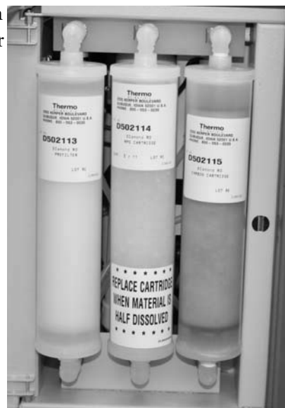
Figure 3-8. Cartridge Installation:(left to right) prefilter, MPS, carbon
